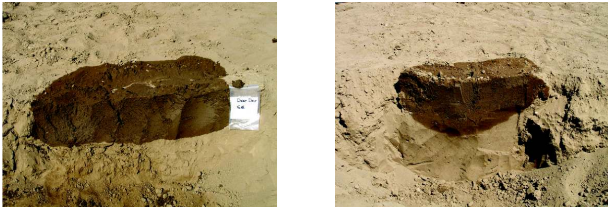
Figure 10. Wetting patterns of surface drip emitters at SE (left) and NW (right) locations
