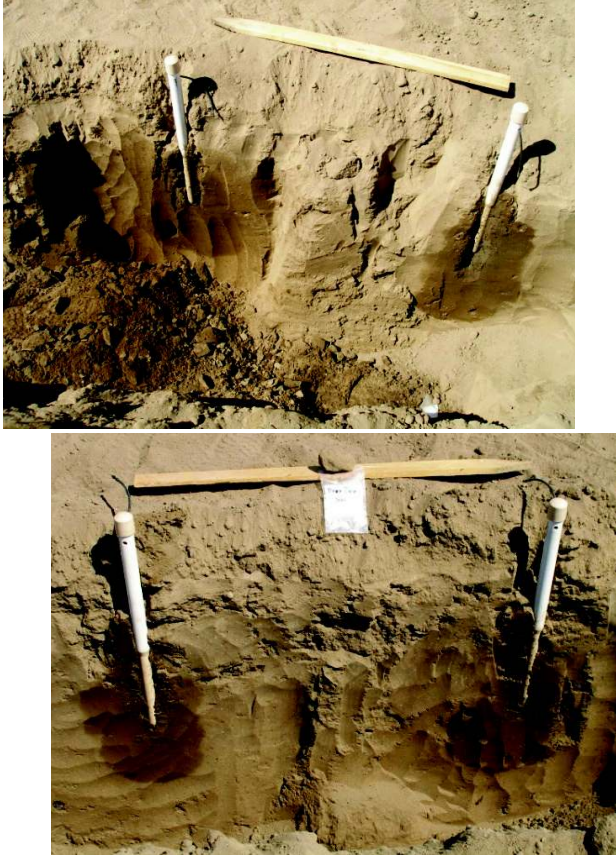
Figure 11. Wetting patterns of Deep Drip™ devices at NE (left) and SW (right) locations
