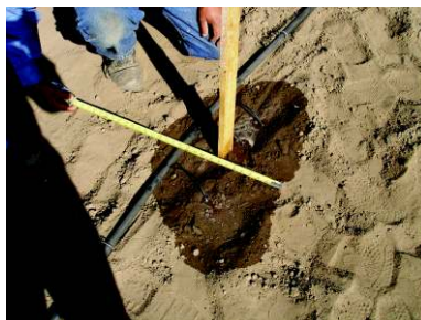
Figure 8. Measurement of wetted width (w) at surface drip location
