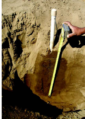
Figure 9. Measurement of wetted depth (z) at Deep Drip™ location
